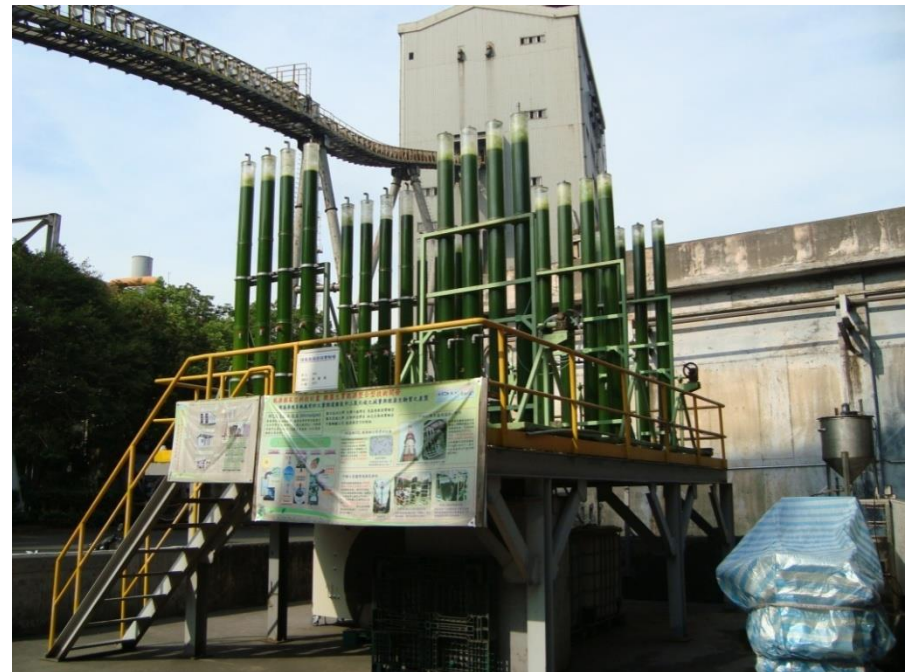
Cultured volume: 40 L/reactor (Total: 6 x 40 = 240 L)
